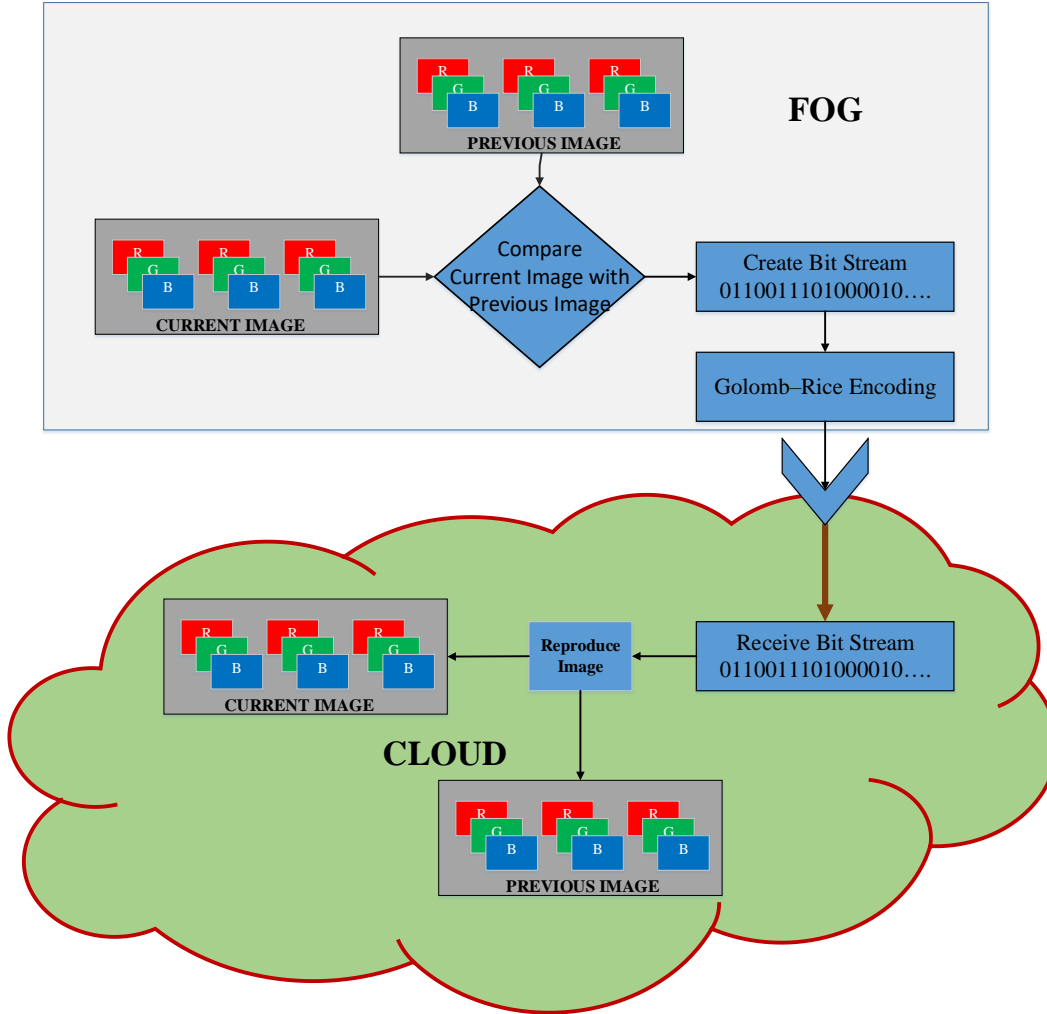
Figure 6.2: Block diagram of the proposed variable length pixel encoding
