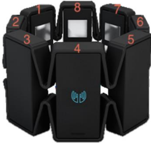
Figure 4-1 8-Channel EMG band (Thalmic Labs, 2015)
