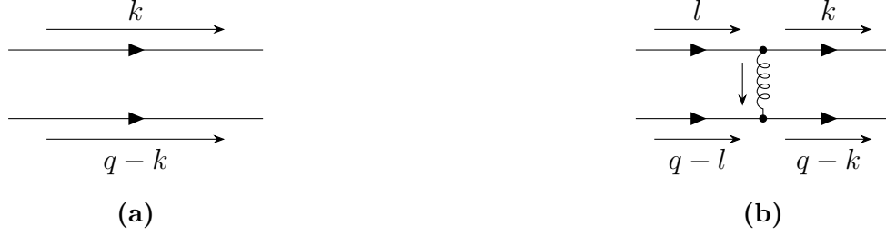
Figure A.2: Feynman diagrams of the LO and NLO of the dipropagator.
